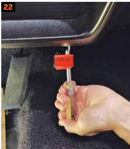
22. Mount the control under the dash, route the cable (and grommet) through your firewall hole.
