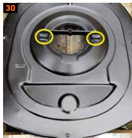
30. The finished product. On this car, we needed to raise the carb strap-bar about one inch, too (circled). You can weld, right?
