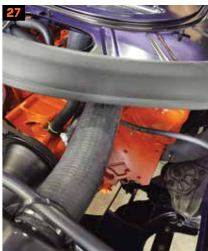
27. The clearance to the upper radiator hose can be snug, if you are not concerned with OEM platinum appearance, adding a sleeve of large convolute tubing is the solution. Hemis had a specially trick curved hose (repros available).
