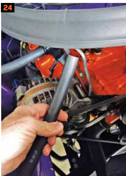
24. Add the drain hoses, trimmed to fit. You're done!
