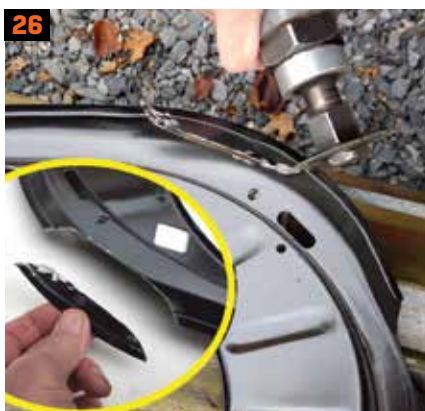
26. First, slice the left rear corner of the adapter ring for clearance as needed. Add primer and the foam seal, and nobody will be the wiser. We've done this hack on 340s and 383s, this hack might be touch-and-go with an RB engine.
