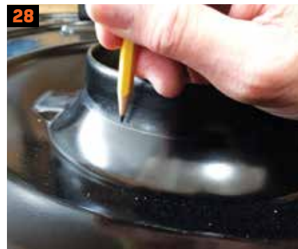
28. What if you have a higher-than-stock manifold? You need to shorten the "funnel" area of the retainer. Measure twice...
