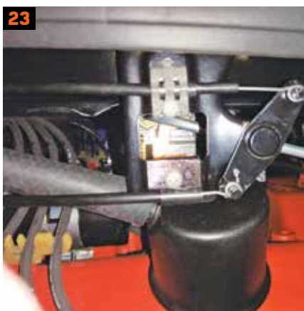
23. Connect both cables to the bellcrank as shown, adjust so fresh air door is fully closed a fraction before the dash knob bottoms.
